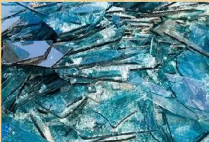
The insertion of shards of recycling in the glass paste allows the use of lower melting temperatures.
