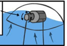
But not all of the energy from the rising wave is used to turn the generator. Some is stored by winding up a counterweight instead. The bigger the wave, the higher the weight is lifted.
