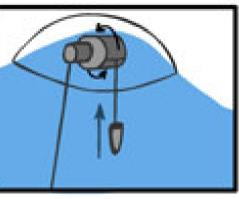
As the wave falls, so does the weight, releasing its stored energy to maintain a constant load on the generator throughout the wave cycle. Energy stored from larger waves can be used to compensate for smaller waves.
