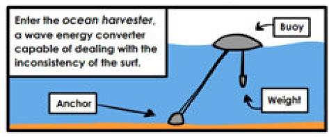
As the harvester rises with a wave, an anchor drum is rotated by the pull of an anchoring wire, driving a generator to produce electricity.
